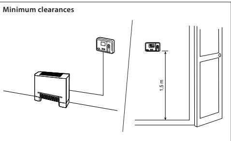
If fitted to a wall, the Room Controller must be mounted:
