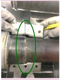
The brazing fillet should be located within the shell groove. Remove the adhesive cap (rotate), replace with the adhesive mixer
