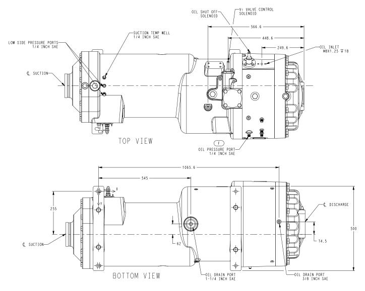
Fig. 3 — Compressor Physical Data and Connections (06ZF, Frame 2) (cont)
