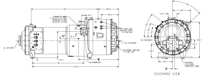
Fig. 3 — Compressor Physical Data and Connections (06ZF, Frame 2)
