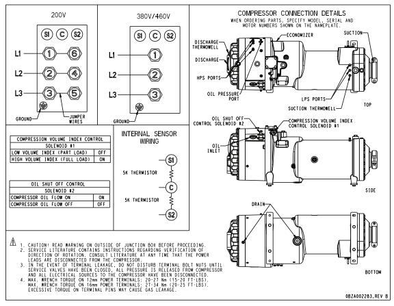
Fig. 13 — Compressor Connection Details
