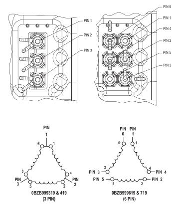
INTERNAL MOTOR LEAD CONNECTIONS
