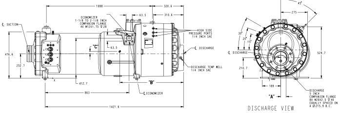
Fig. 4 — Compressor Physical Data and Connections (06ZJ, Frame 3)
