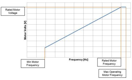
Fig. 14 — Sample Compressor Motor Voltage Curves
