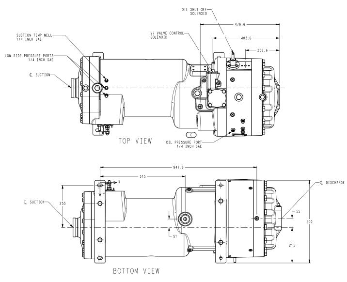
Fig. 2 — Compressor Physical Data and Connections (06ZC, Frame 1) (cont)
