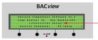
Fig. 11 — Controller Setup Menu
